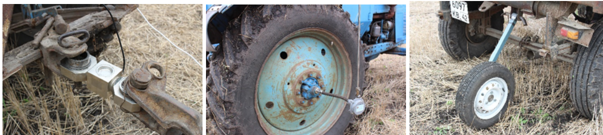
(b) strain gauge sensor for measuring tractive effort K-R-20G-20-C1 (c) sensors of driving wheel revolutions on the tractor IP-268 (d) distance traveled sensor IP-266
